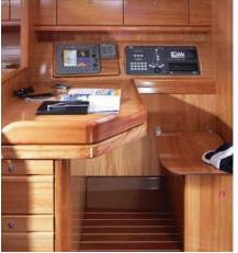
• The Cruiser series' chart table has a large compartment for nautical charts and navigation instruments, with additional stowage beneath the seat.
